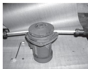
4) Use screwdrivers to detach the impeller.
