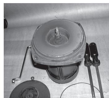
6) The motor unit is without an impeller. Replace the shaft seal when necessary (see Replacing a shaft seal).
