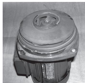
2) Install the motor unit in a vertical position.
