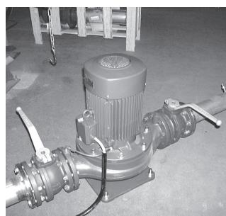
2) Close the valves and detach the connecting cable of the motor. Next, detach the flush pipe (in ALH pumps). Open the screws/bolts of the operation unit.
