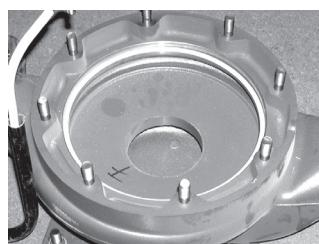
4) Replace the gasket/O-ring of the housing.
