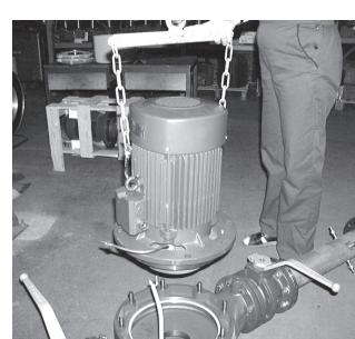
3) Lift the operation unit by means of a hoist. Watch out for hot water!
