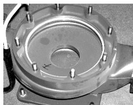
4) Replace the gasket/O-ring of the housing.
