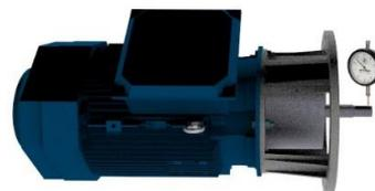
10) Align flange-shaft using a measuring gauge. The max. allowed run-out is 0.08.
