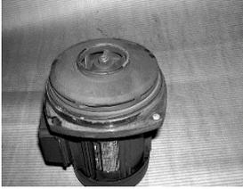
3) Open the screw/nut of the impeller.
