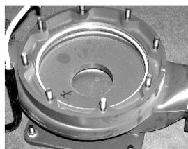
4) Replace the gasket/O-ring of the housing.
