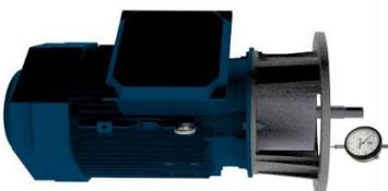
11) Align the flange perpendicularity run-out to motor shaft using a measuring gauge. The max. allowed run-out is 0.15.
