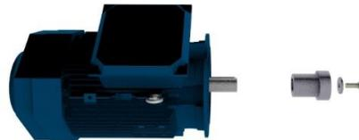
8) Detach coupling from the motor shaft.
