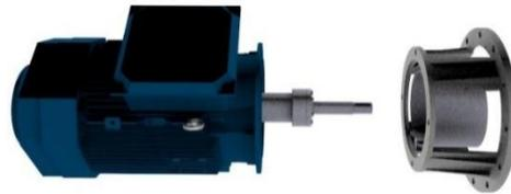
6) Detach motor bracket (adapter) from electric motor.
