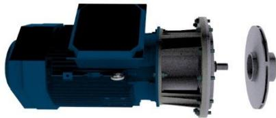
3) Open the screw/nut of the impeller. Use an extractor if necessary.
