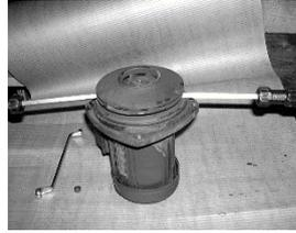
4) Use screwdrivers to detach the impeller.
