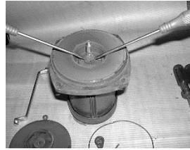
2) Detach the shaft seal using two screwdrivers. Do not damage the sealing surface of the shaft.
