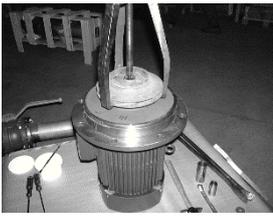
5) Use an extractor if necessary. Pull out the impeller at the impeller wings.
