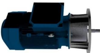
9) Install coupling, flange-shaft and motor bracket to new motor. Use threadlocker Loctite 2701.
