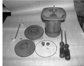
4) The motor unit disassembled, with installation tools.
