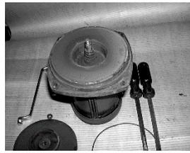
6) The exchange unit is without an impeller. Replace the shaft seal when necessary (see 16. Replacing shaft seal).
