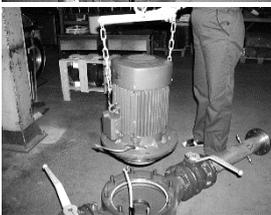
5) Install a new exchange unit. Tighten the screws/nuts of the unit evenly.
