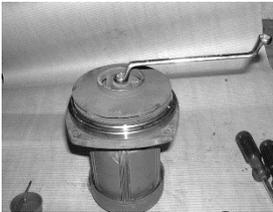
7) Install a new impeller. If required, you can lightly tap the impeller with a rubber mallet until flush with the ridge. Tighten the screw/nut of the impeller.
