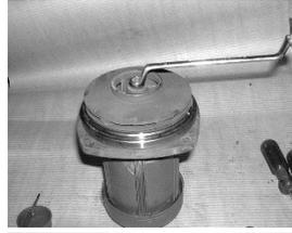
2) Install the exchange unit in a vertical position.
