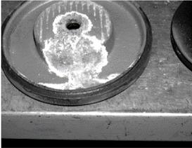
3) Also detach the sealing flange from the motor front plate using two screwdrivers. If needed, replace the sealing flange with a new one.
