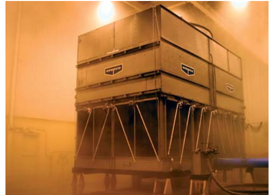
The Research Center includes state-of-the-art Thermal Test Chambers for testing and evaluation of full-scale evaporative cooling and heat transfer equipment.
